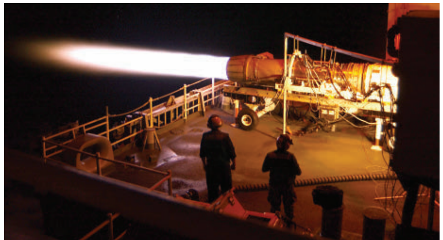
Military personnel harness Astronics Test Systems equipment to test jet engines on an aircraft carrier.
